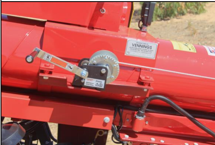
Optional winch adjustable allows the hopper to be raised & lowered without climbing under silo
