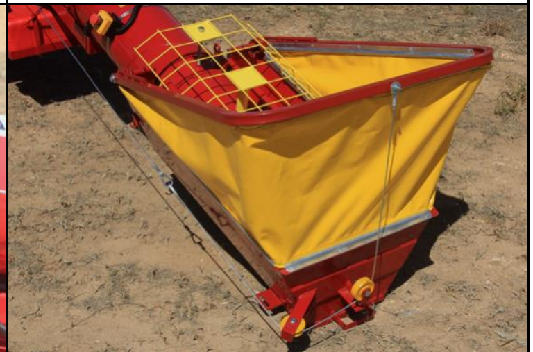
Hopper in raised position with wire rope & pulleys.
