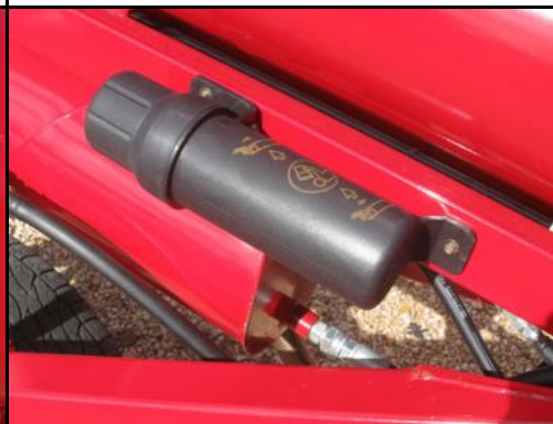
Document holder attached to Auger holds motor and auger operating instructions
