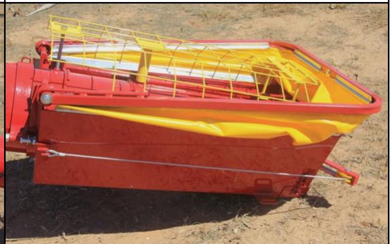
Hopper collapsed ready for transport wire rope holds the hopper down.
