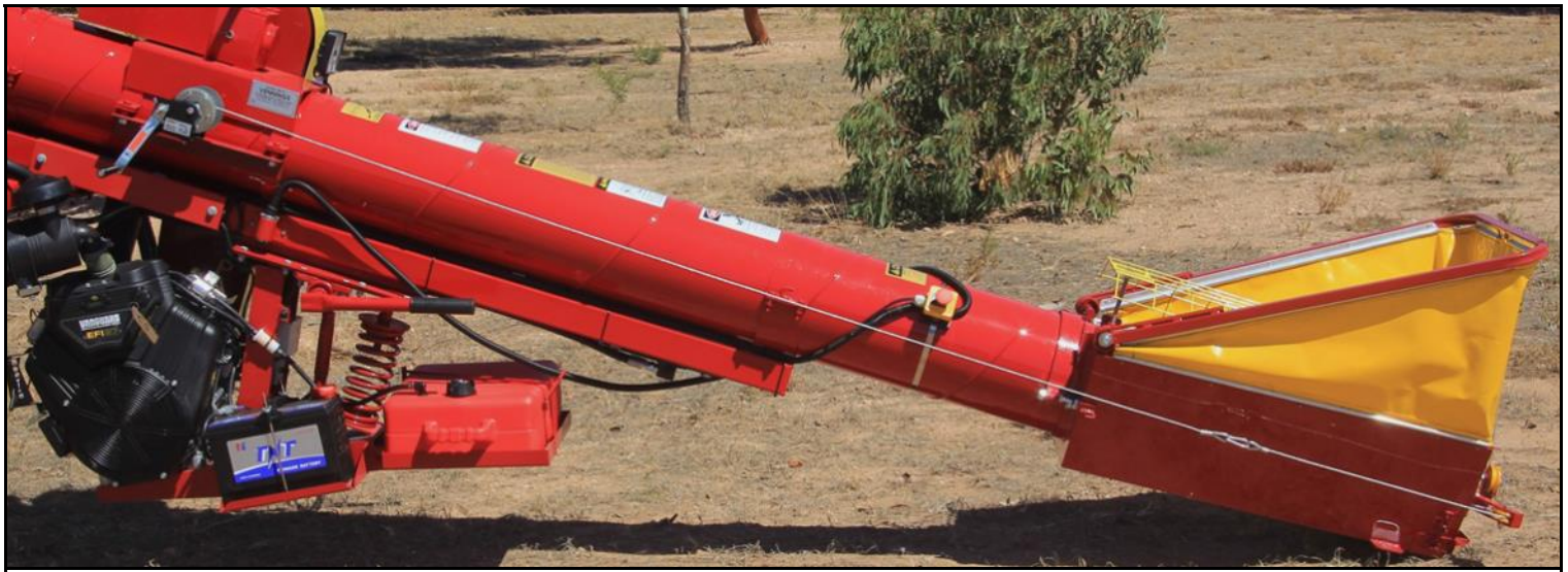
Winch adjustable collapsible hopper in raised position. Simply wind the winch to collapse the hopper into its lowered position
