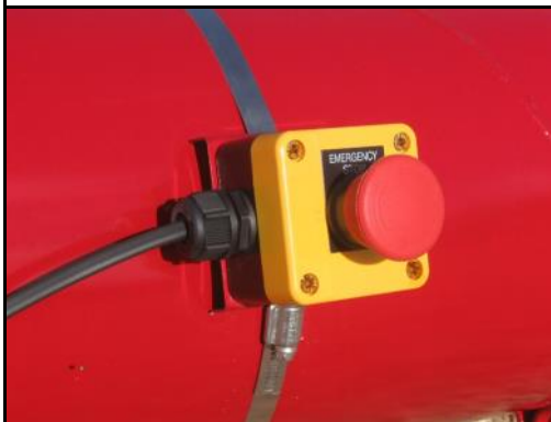
Emergency Stop Switch fitted near intake end of auger
