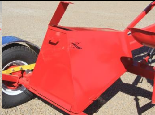
Steel hopper in transport position mounted to bottom frame so its always with auger.
