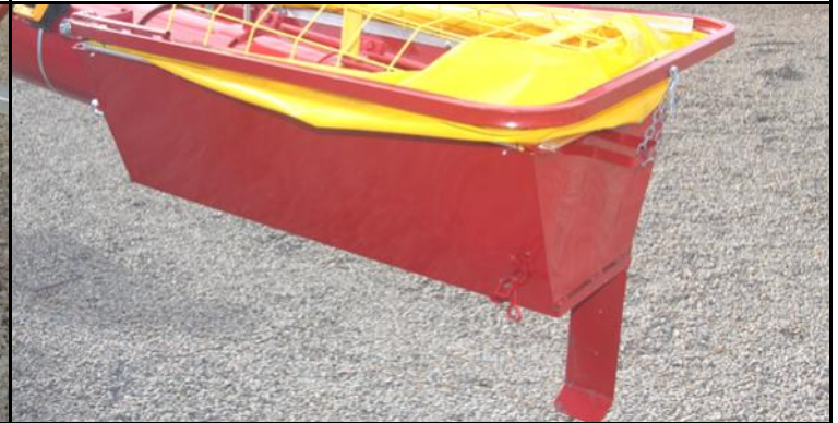
Cleanout trapdoor on bottom of hopper
