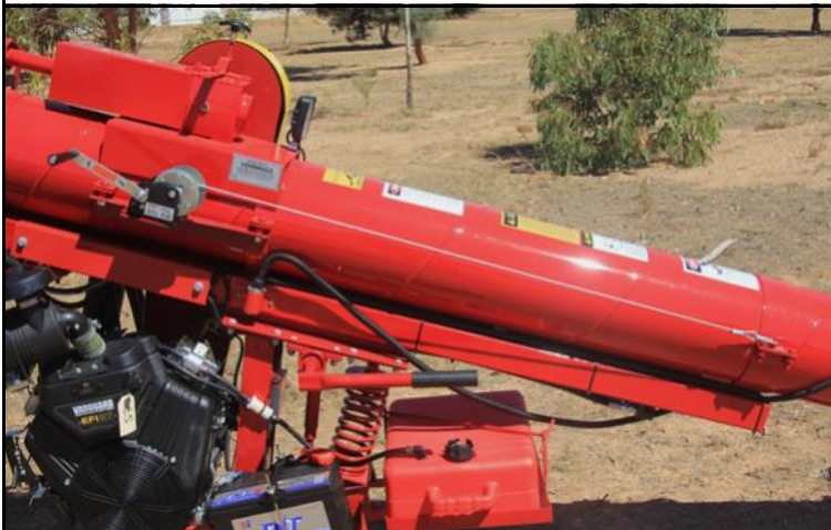
Winch and wire rope in transport position. Winch and Hopper have two separate ropes
