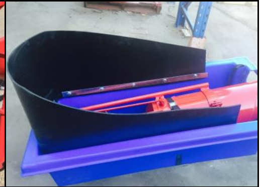
Poly Hopper with rubber top. Slender design allows auger to be placed under silo with the hopper attached to the auger.
