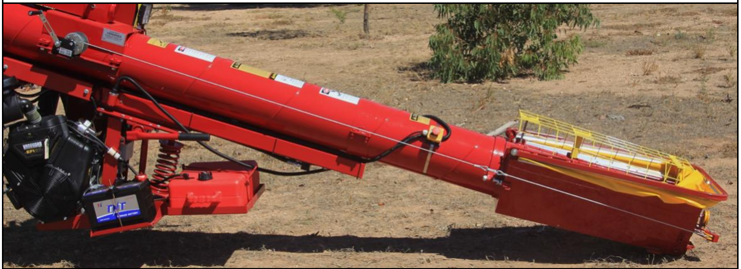
Winch adjustable collapsible hopper in lowered position
